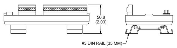
Figure 3-5: I/O Expansion Module Dimensions
